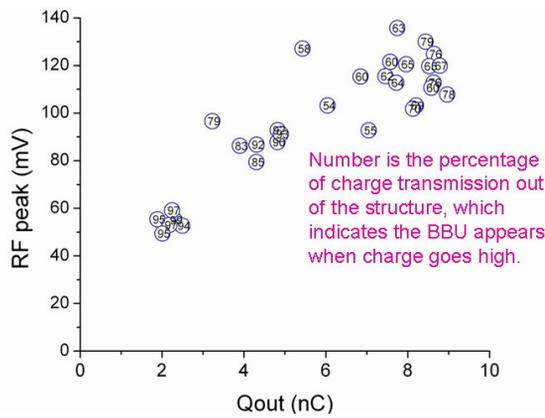
Figure 5: The measured rf signal strength in the scope increased with the transported charge (charge measured out of the power extractor). The bunch train consisted of 4 bunches.
