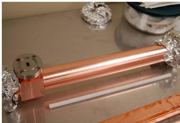
Figure 1: Fabricated 26 GHz dielectric-based wakefield power extractor and dielectric (consisting of three 10-cm long dielectric tube segments) prior to loading.
