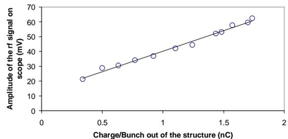
Figure 4: The measured rf signal strength in the scope increased linearly with the transported charge. The bunch train consisted of 16 bunches.
