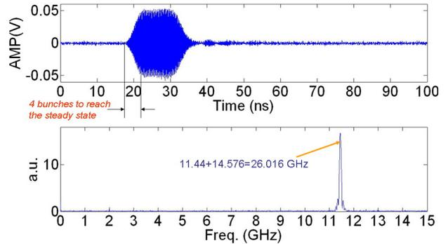
Figure 3: The down-converted rf signal and its frequency spectrum obtained in the beam test of the 26 GHz wakefield power extractor. A 14.576 GHz local oscillator was used to down-convert the signal. A bunch train consisting of 16 bunches was used.
