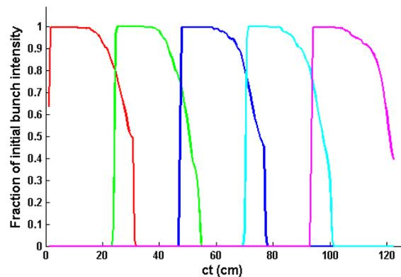
Figure 6: Intensity vs. time for the five bunch simulation. Different color represents different electron bunch in a bunch train.
