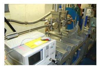
Figure 1: The new AWA RF gun (behind the blue solenoid) will replace the present drive gun. The two gate valves, and the long actuator connected to the back side of the gun, allow the insertion of the Cesium Telluride photocathode without exposing it to air.
