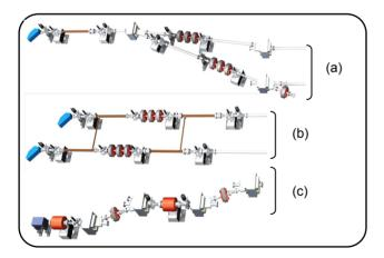
Figure 4: Different legs of the new AWA beamline switchyard will be dedicated to specific types of experiments: (a) collinear wakefield acceleration; (b) two-beam-acceleration and RF power generation; (c) phase space manipulation (emittance exchange) and beam diagnostic development.
