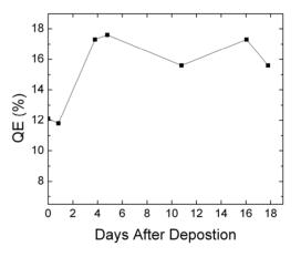
Figure 2: Cesium Telluride quantum efficiency: (a) time evolution during Cesiation in the fabrication chamber. The curves correspond to three depositions made at different rates; (b) lifetime of photocathode kept in preparation chamber for eighteen days. The quantum efficiency can show a slight increase in the initial few days, but typically it will start decreasing after a few weeks.
