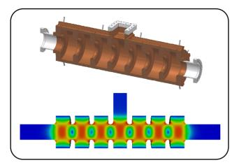
Figure 3: CAD rendering and field map of the new AWA linac tanks. The 3D numerical simulation was performed with Omega3p.
