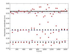
Figure 2: Horizontal coordinates (red squares) read by 84 BPMs in EMMA. The distortion in the signal is due to horizontal magnet misalignments with 50 microns sigma. The three groups represent the three locations of BPMs in the EMMA cell (see Fig. 1). The black squares represent the ideal closed orbit. The dashed blue line is the target orbit found by averaging the BPM signals.
