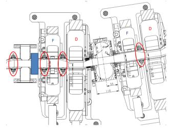
Figure 1: Two EMMA cells highlighting the location of the BPMs (circled in red) and the vertical corrector magnet (blue square). The two leftmost BPMs are at either end of a long drift.
