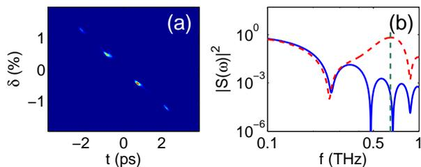
Figure 3: Simulated longitudinal phase space ( $t, \delta$ ) downstream of the EEX beamline (a) and resulting bunch form factor [red trace in plot (b)]. The blue trace in plot (b) is the bunch form factor computed for the entire beam (360 pC) at X24 i.e. when the X3 slits are not inserted. In image (a)  $t > 0$  corresponds to the tail of the bunch.
