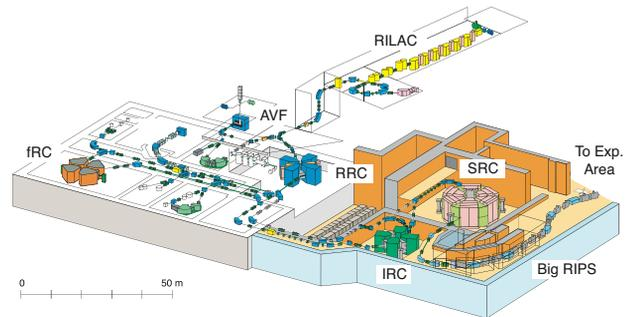
Figure 4: Layout of the accelerator complex of RIKEN RIBF.
