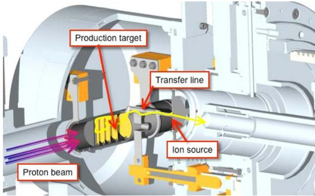
Figure 8: Schematic drawing of the target developed for the SPES project.
