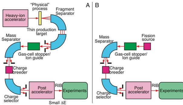
Figure 3: Catcher-reacceleration scheme (A) and direct scheme starting with fission source (B).
