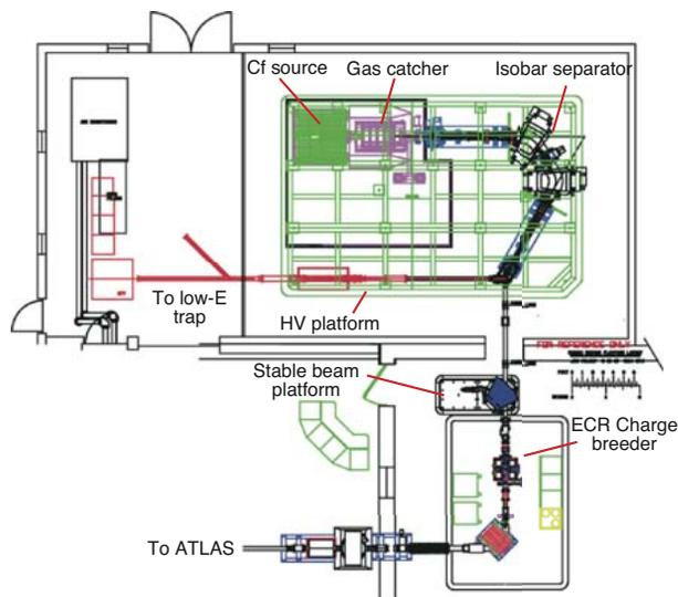
Figure 6: Floor plan of CARIBU project at the ATLAS facility, ANL.
