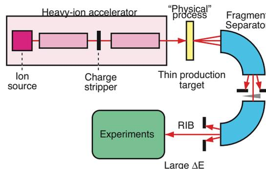
Figure 1: Schematic drawing of the in-flight production method.
