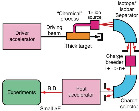
Figure 2: Schematic drawing of the ISOL production method.
