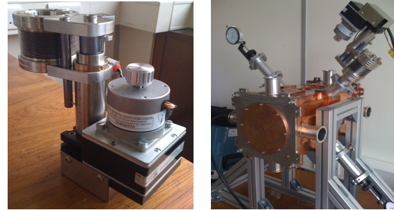
Figure 1: The tuner stepper motor with welded bellow alone, and fitted on the RFQ cold model.
