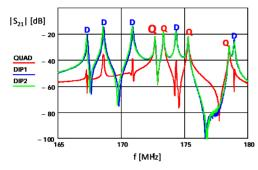
Figure 2: Mode spectra of the Aluminum RFQ.
