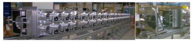
Figure 1: The aluminium model of the IFMIF RFQ set up for measurements at LNL (left) and the bead pulling system (right).
