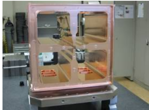
Fig.4: The RFQ prototype module after the first brazing step.
