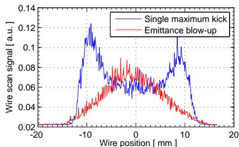
Figure 3: Vertical transverse beam profile at the wire scanner location after one single kick at the maximum kicker strength (blue) and after slow emittance blow-up (red). The typical hollow beam shape is clearly visible. The maximum aperture seen with the slow blow-up is about 1 mm more, as seen in the small tail at position -15 mm.
