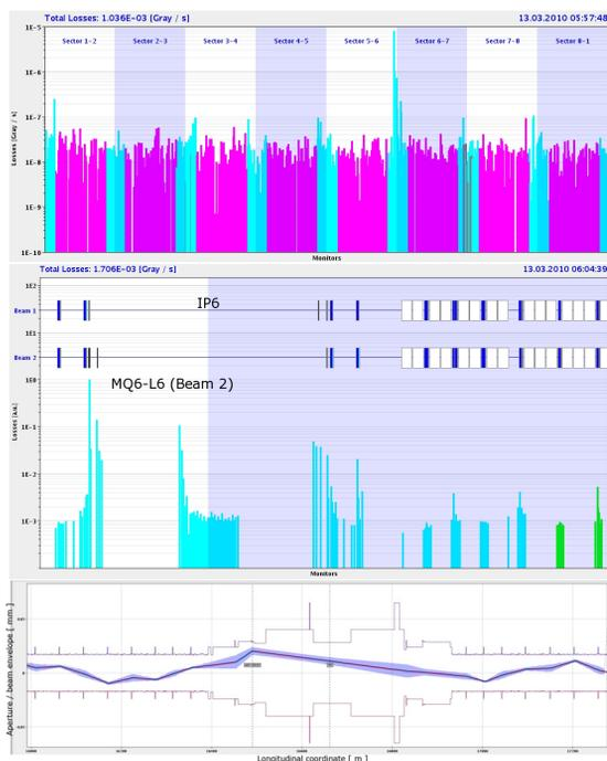
Figure 2: Beam losses around the ring (top) and in IP6 (middle) and beam orbit during a global aperture scan. The main bottleneck is the quadrupole Q6-L6. Secondary loss peaks appear at other location due to the scattering at the primary loss location.
