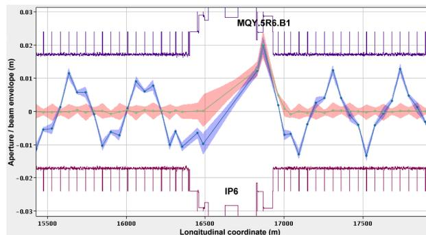
Figure 1: Examples of closed-orbit oscillation for global aperture measurements (blue) and local orbit bumps (red), with a  $3\sigma$  beam envelope. The aperture model uses detailed measurements of the cold magnet profiles every 10 cm.
