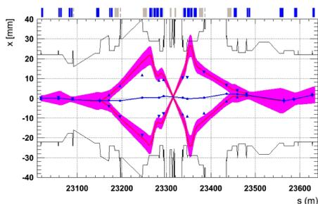
Figure 5: Local aperture bump in IP8 (LHCb).
