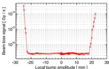
Figure 4: Beam losses versus amplitude of orbit bump during a local scan at the quadrupole MQY-4L6-B1. Beam losses are measured with BLMs installed on the quadrupole and increase as the beam is lost on the magnet aperture. Note that the loss values at the two bump sides depend on the amount of beam that is cut.
