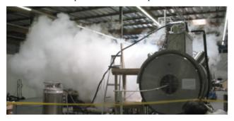
Figure 7: Quench during spectrometer solenoid training.
