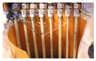
Figure 6: Burned out HTS lead (right side).
