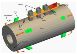
Figure 3: Overall view of the first stage thermal model.
