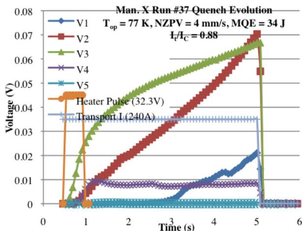
Figure 5: Voltage response of Man. X quench test Run 37.
