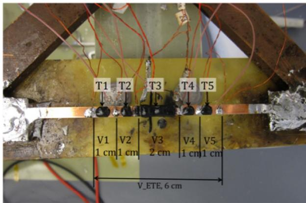
Figure 2: Experimental set-up for Man. X GdBCO conductor
