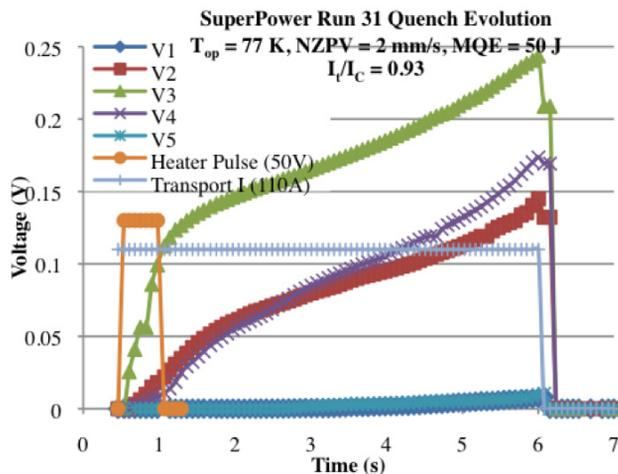
Figure 4: Voltage response of SuperPower quench test Run 31.
