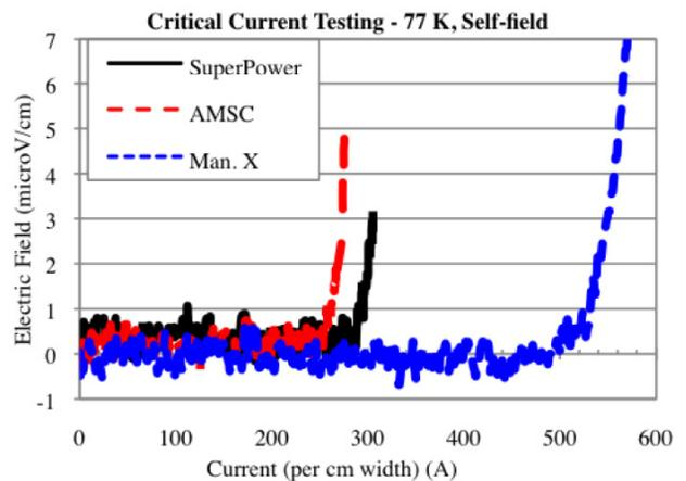
Figure 3: E-I curve for three REBCO conductors at 77 K.
