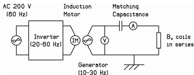
Figure 4: Schematic measurement set-up of AC losses of the  $B_x$  coils at 20 K. Details are described in the text.
