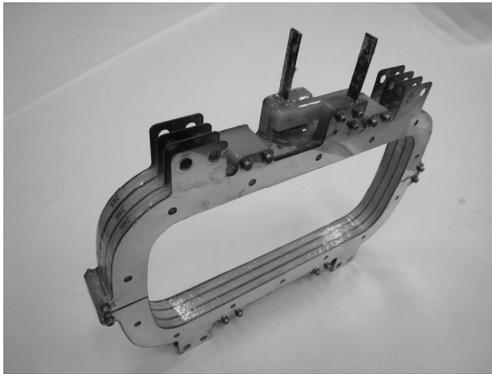
Figure 2: Photograph of single assembled  $B_x$  coil.
