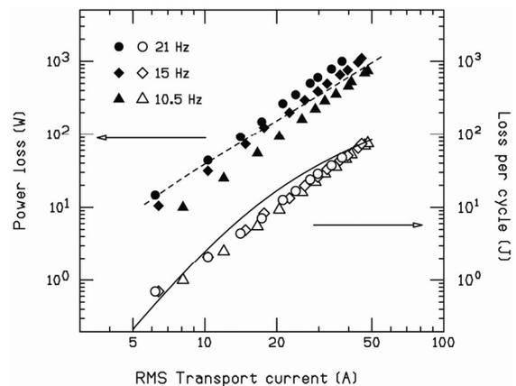
Figure 5: Measured AC losses at 20 K of the  $B_x$  coils in series. Full symbols show the total power losses on the left side scale. Open symbols present losses per cycle on the right side scale. The dashed curve shows the model calculation by King [11]. The solid curve is a theoretical prediction normalized to the measured data.
