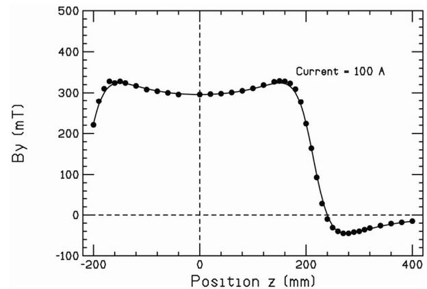
Figure 3: Dark points represent measured  $B_y$  fields along the central axis at 100 A. The solid curve shows the calculated magnetic field.
