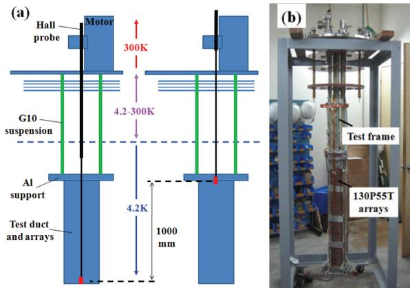
Figure 2: (a) and (b) display the assembly of arrays and measurement system in the vertical dewar.
