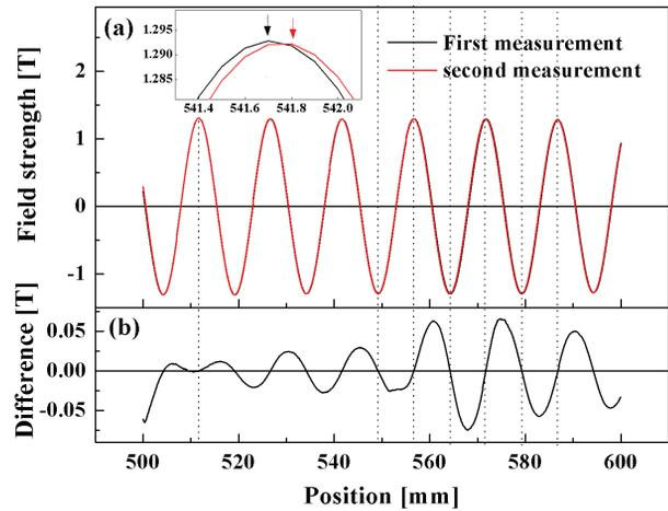
Figure 4: (a) plots the tests of the reproducibility of position and amplitude of the Hall probe. Figure 4(b) plots the difference spectrum of both scans.
