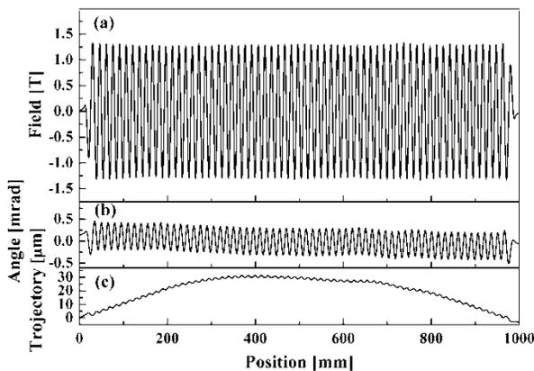
Figure 3: (a), (b) and (c) are plot the measured field spectra, angle and trajectory at 458 A, respectively.
