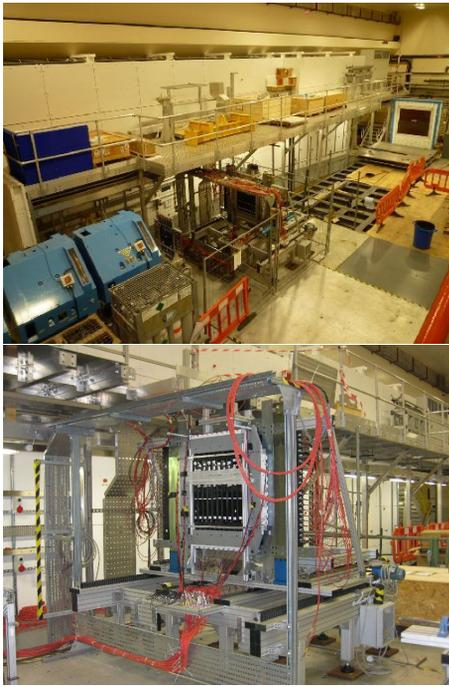
Figure 3: Top panel: presently installed beamline in the MICE Hall at RAL. TOF1 is on the temporary trolley and TOF2 on the final downstream RM3 platform in front of KL. Bottom panel: enlargement of TOF2 and KL.
