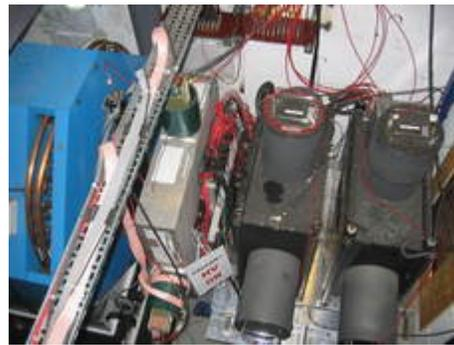
Figure 2: Image of TOF0 and the two Aerogel Cerenkov counters in final position inside the closed DSA area at RAL. Beam impinges from the left.
