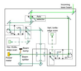
Figure 3: Schematic layout of the vertical breadboard.
