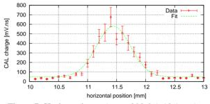
Figure 7: Horizontal scan ( $\sigma_x = 293.6 \pm 18.1 \ \mu m$ ).
