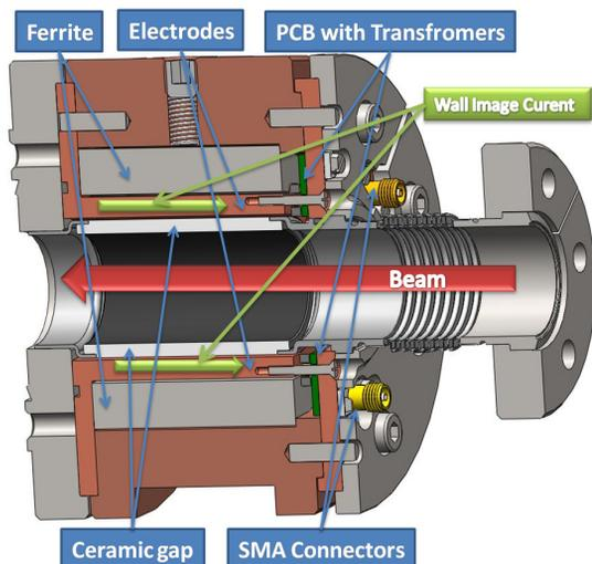
Figure 2: Cross section of a BPS monitor showing the wall current flow.
