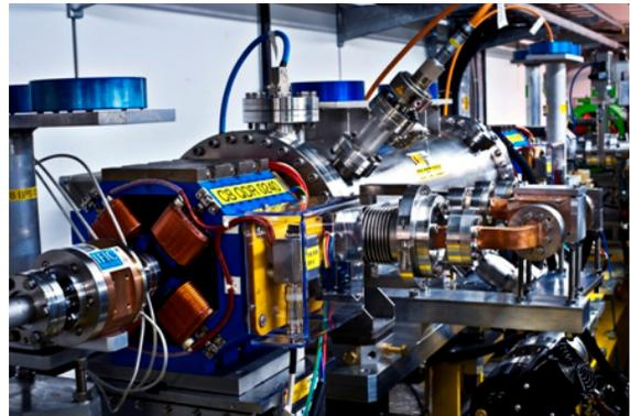
Figure 1: View of a PETS tank, a quadrupole and a BPS in TBL line at CLEX area.
