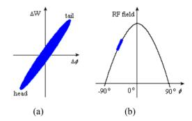
Figure 1: Energy chirping in longitudinal phase space (a) and RF phase in accelerating column (b).
