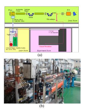
Figure 4: Layout of PAL fs-THz facility (a) and view of linac tunnel (b).
