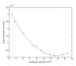
Figure 5: The result of quadrupole scanning method for emittance measurement.
