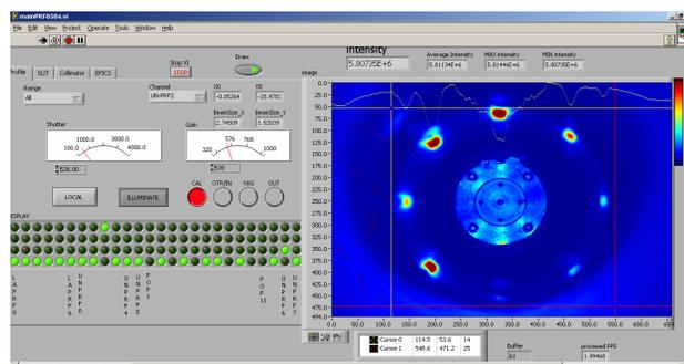
Figure 3: Beam Profile Diagnostic Control Panel in LabVIEW.
