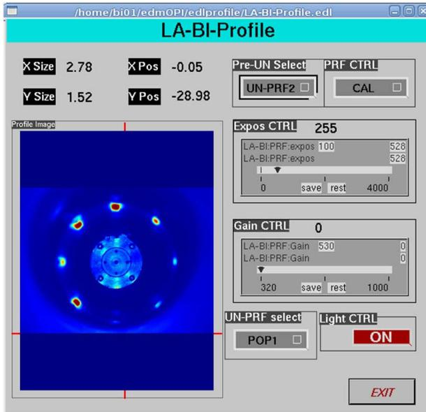
Figure 4: Beam Profile Diagnostic Control Panel in EDM.
