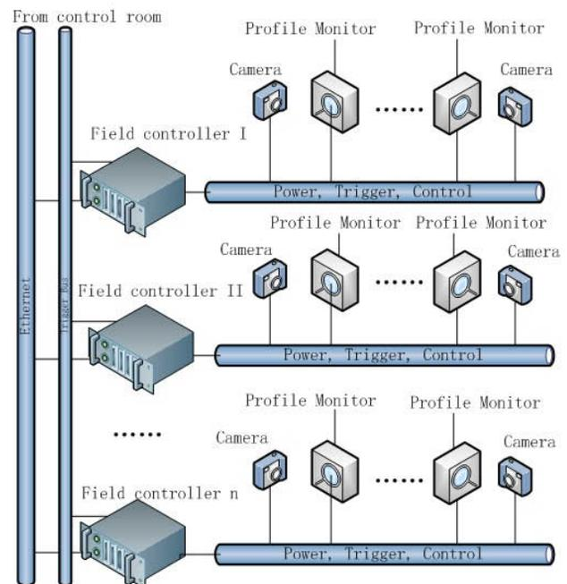
Figure 2: Structure of the beam profile diagnostics system.
