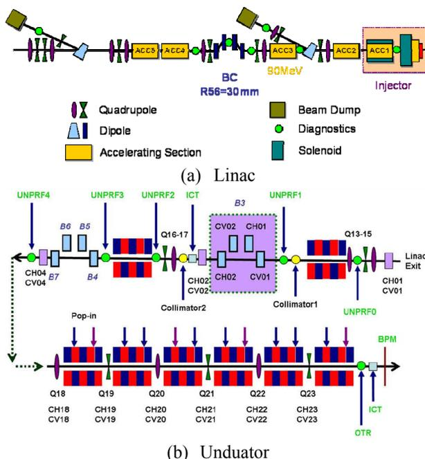
Figure 1: Layout of SDUV-FEL.
