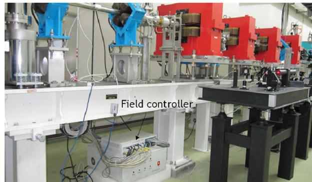
Figure 7: Beam profile diagnostics controller in the field.
