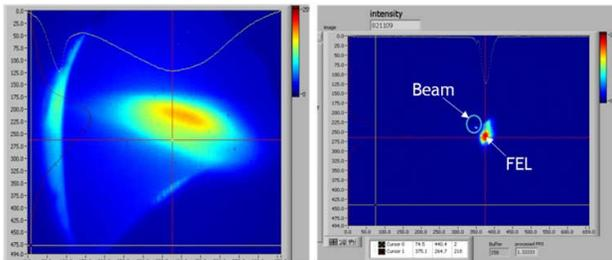
Figure 5: Images from the Pop-in monitor and the profile monitor.
