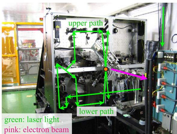
Figure 1: Optical table of the Shintake monitor
