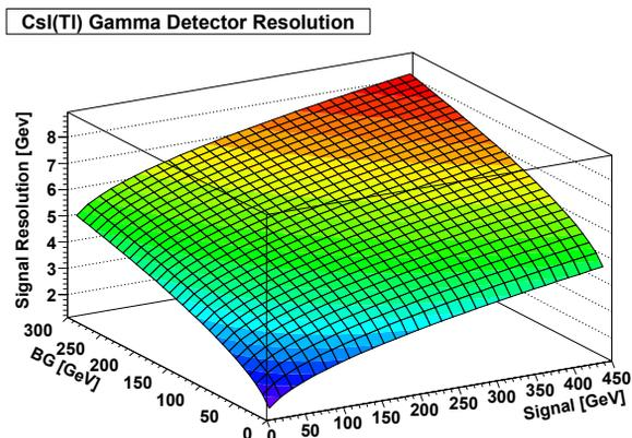
Figure 3: Simulated resolution of the gamma detector
