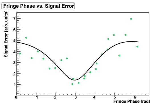
Figure 4: Relation between signal error and the fringe phase measured by beam size measurement
