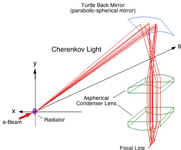
Figure 2: Schematic apparatus of the LFC-camera. The system consists of a specific (parabolic-spherical) mirror and two aspherical condenser lenses. Angular distribution of the Cherenkov radiation is imprinted onto a straight focal line.
