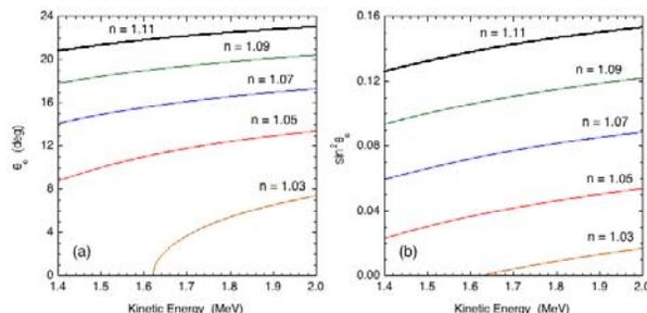
Figure 1: (a) The Cherenkov angle and (b) the value of  $\sin^2 \theta_c$  for various refraction indexes, plotted as a function of the kinetic energy.
