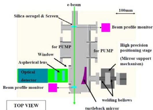
Figure 4: Configuration of the LFC-camera. The turtleback mirror is supported by high precision positioning mechanism. Silica-aerogel is placed in the holder.
