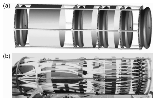
Figure 2: (a) Schematic view of a tracker. Five stations are installed with optimized spacing. Light-guides are not shown. (b) A photograph of the upstream tracker with internal light-guides installed.
