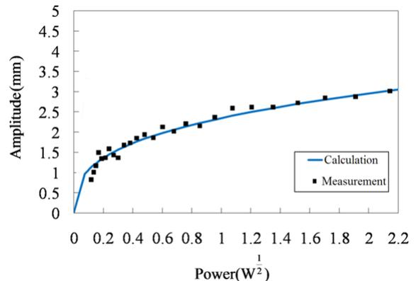
Figure 4: Measured and calculated horizontal betatron oscillation amplitude as a function of applied power.
