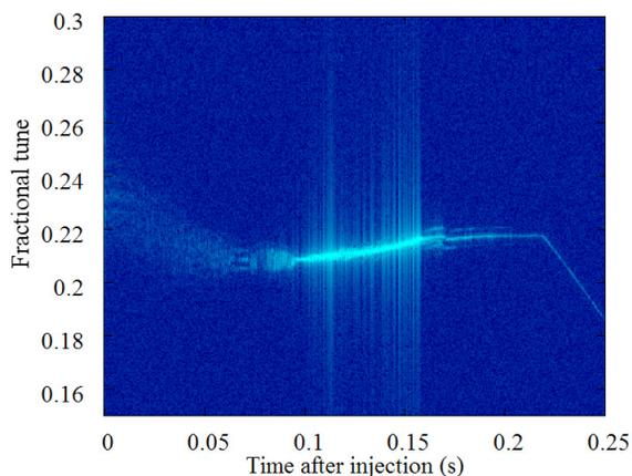
Figure 6: Measured betatron tune of the UVSOR-II booster synchrotron as a function of time after injection. In a usual operation, electron beam is extracted from the booster synchrotron before the changing point of 0.22 sec.
