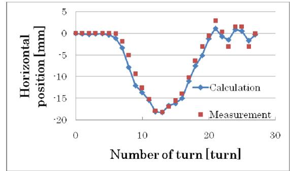
Figure 3: Measured bump orbit compared with numerical calculation.
