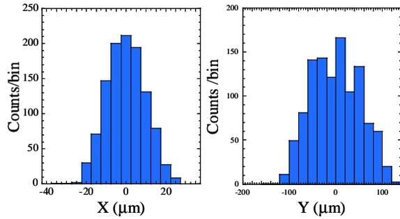
Figure 2: Accuracy of turn by turn BPM system (left shows horizontal right shows vertical).
