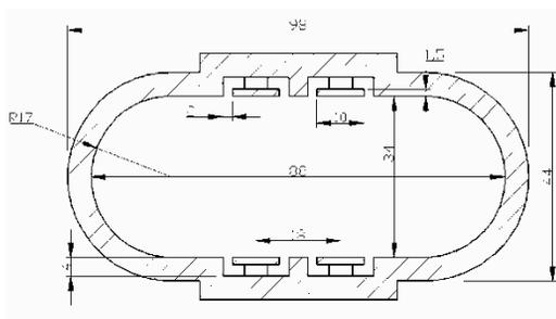
Figure 5: Cross section of RF knockout chamber designed for tune measurement.
