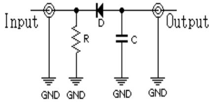
Figure 1: Diagram of wave processing circuit for turn by turn BPM.
