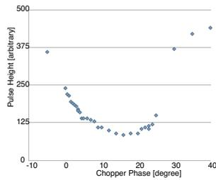
Figure 6: Chopper inefficiency vs. Phase
