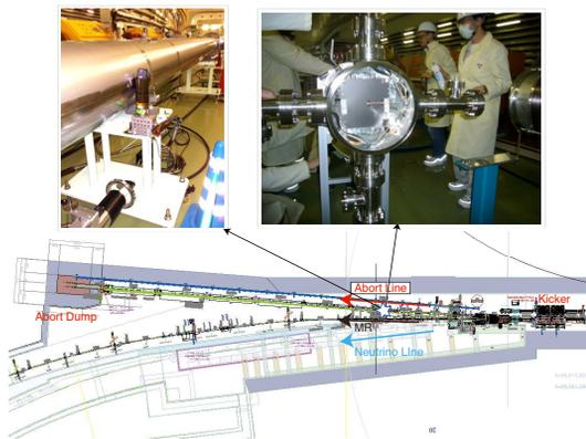
Figure 3: Beam monitors used for abort line measurements.
