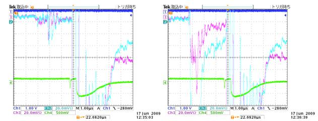
Figure 5: Beam leakage observed in the flying wire measurement. (Left:FWPM OFF, Right:FWPM ON)
