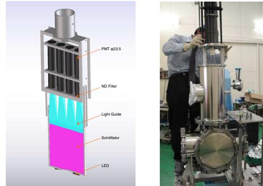
Figure 8: New extinction monitor.
