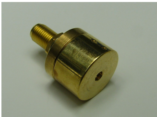
Figure 3: TRIUMF built single crystal diamond detector for the purpose of low intensity diagnostics.
