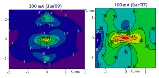
Figure 1: Contour plots of drag rates measured for  $I_e = 0.3$  A (left, interpolation from 30 points measured across the beam) and 0.1 A (right, 14 points), both with no ion clearing by interruptions. Contour levels are in MeV/c/hr.
