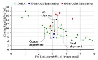
Figure 2: Longitudinal cooling rate measured in 2006-2010. The arrows connect points measured on the same day to show the range of several improvements. All measurements are "on axis".
