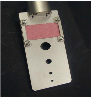
Figure 4: The orbit correction slit plate for the beam and the cooling laser. Alumina fluorescent plate and the hole of  $\phi 10, 6, 3, 2$ mm has been installed on the stainless plate. Aperture size is adjusted by using the lower side of a stainless plate.
