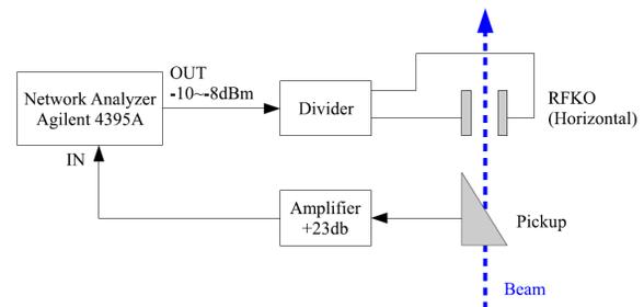
Figure 3: Conceptual diagram of Measurement of beam transfer Function
