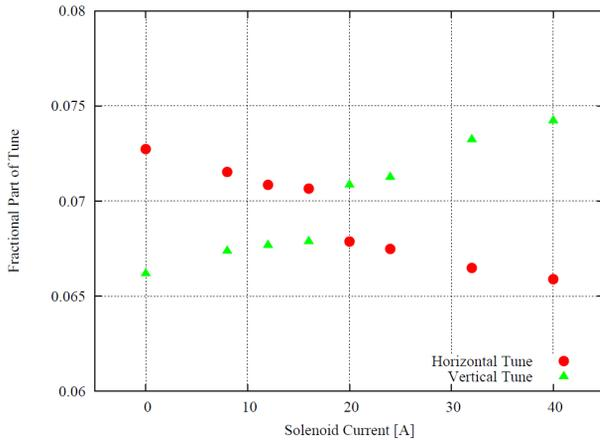
Figure 4: Solenoid current dependency of horizontal and vertical betatron tunes
