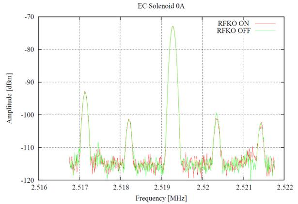
Figure 5: Signal of vertical oscillation (Solenoidal Current: 0 A)
