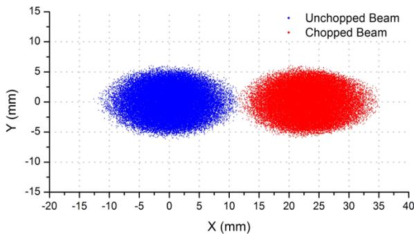
Figure 3: Chopped (red) and unchopped (blue) beam separation in the transverse plane at the end of the fast chopper beam dump.
