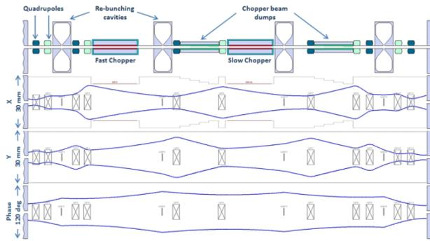
Figure 2: Beam envelopes in the MEBT line (transverse and longitudinal planes) with the beam choppers switched off (from TraceWin/Partran).
