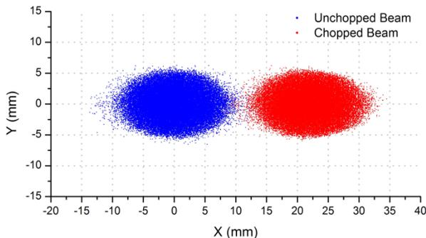
Figure 4: Chopped (red) and unchopped (blue) beam separation in the transverse plane at the end of the slow chopper beam dump.
