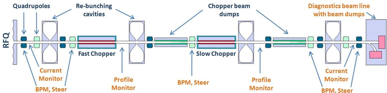
Figure 1: Schematic drawing of the FETS MEBT line with diagnostics (~4.5m long).
