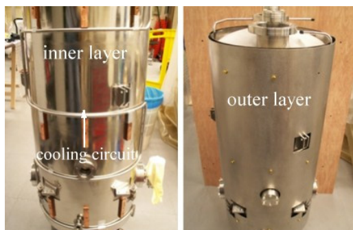
Figure 6: MB14 cavity equipped with its dual-layer magnetic shield.
