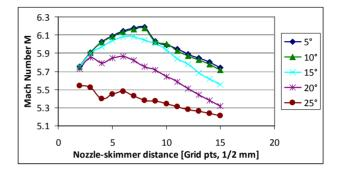
Figure 3: Mach number plotted as a function of nozzleskimmer distance, with the aperture angle  $\alpha$  as parameter.
