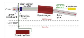
Figure 2: Overview of the laser-wire setup.
