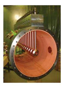
Figure 4: DTL prototype.
