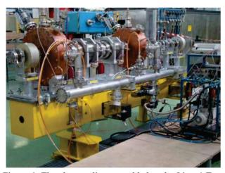
Figure 6: The chopper line assembled at the Linac4 Test Stand.
