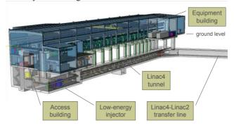
Figure 2: The Linac4 installations.
