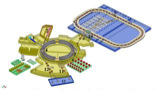
Figure 1: Scheme of NICA facility: 1 – light and polarized ion sources and "old" Alvarez-type linac; 2 – ESIS source and new RFQ linac; 3 – Synchrophasotron yoke; 4 – Booster; 5 – Nuclotron; 6 – beam transfer line; 7 – Nuclotron beam lines and fixed target experiments (to be dismantled); 8 – Collider; 9 – MPD; 10 – SPD; 11, 12 – transfer lines; 13 – new research.
