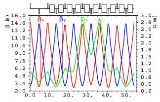
Figure 3: Betatron and dispersion functions for one SP.
