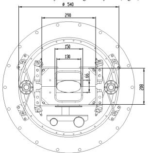
Figure 5: Cross-section of the dipole magnet in cryostat.
