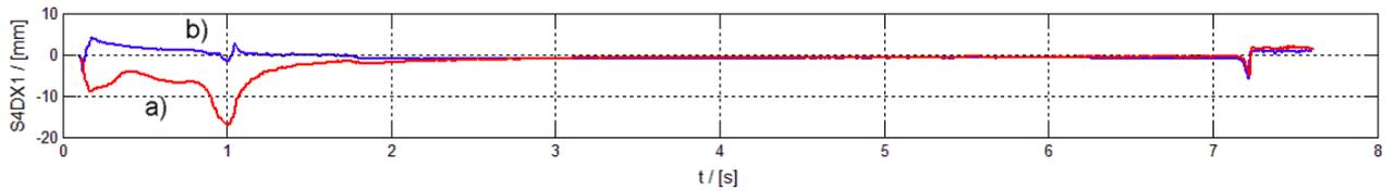
Figure 2: Radial deviation of the beam position without field control (a) and with field controlled (b) magnet currents.
