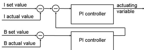
Figure 4: Block diagram of the overlay control loop.
