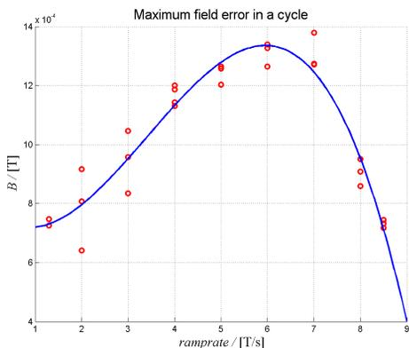
Figure 5: Maximum field error at the end of the ramp. Line is to guide the eye.
