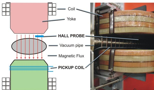
Figure 3: Sensors in a synchrotron dipole.
