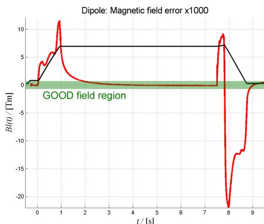
Figure 1: Magnetic field of a synchrotron dipole (black) with the magnetic field deviation x1000 (red).
