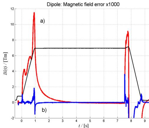
Figure 6: Magnetic field and deviation x1000 (red) without (a) and with field control (b).
