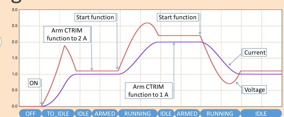
The IDLE, ARMED and RUNNING states are used by the CERN LHC converter controllers to run functions synchronously on demand.
