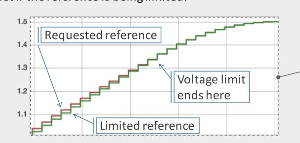
If the reference from the previous iteration was clipped, the time offset is adjusted so that the clipped reference would have been generated.
