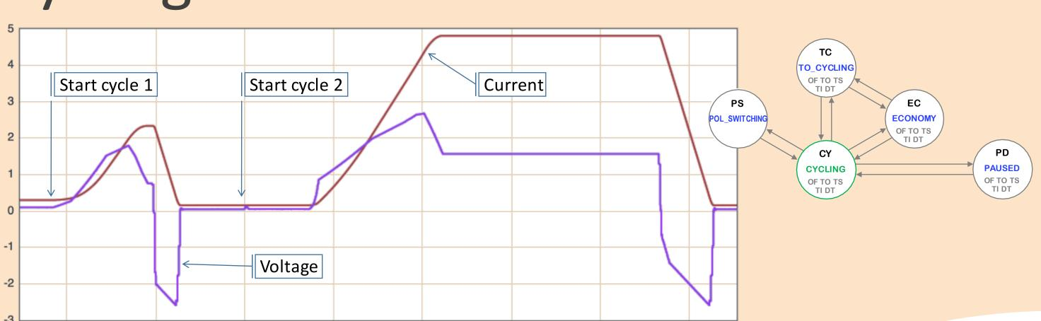
The CYCLING state is used for fast cycling accelerators. Reference functions are armed in advance. The real-time selection of functions is made by the timing system.
