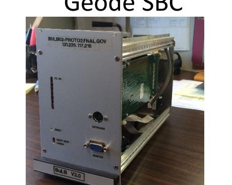
PC/104 Integrated in NIM module
