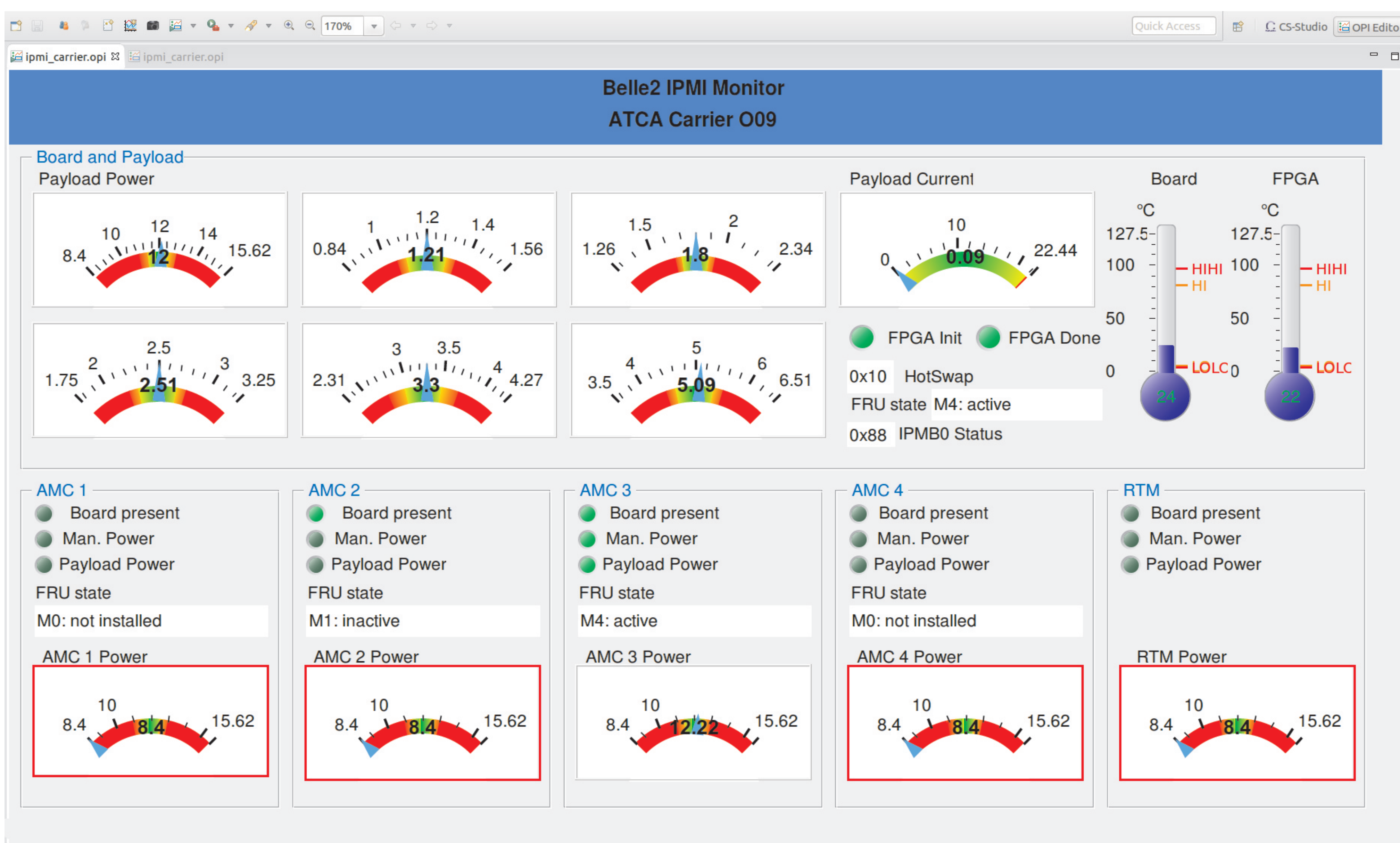
CSS showing an OPI with sensor readings from an ATCA Carrier Board.
