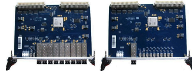
Fig. 5: The EVG (event generator) and EVR (event receiver) in timing system, which is provided by Shanghai institute of applied physics, Chinese Academy of Sciences.
