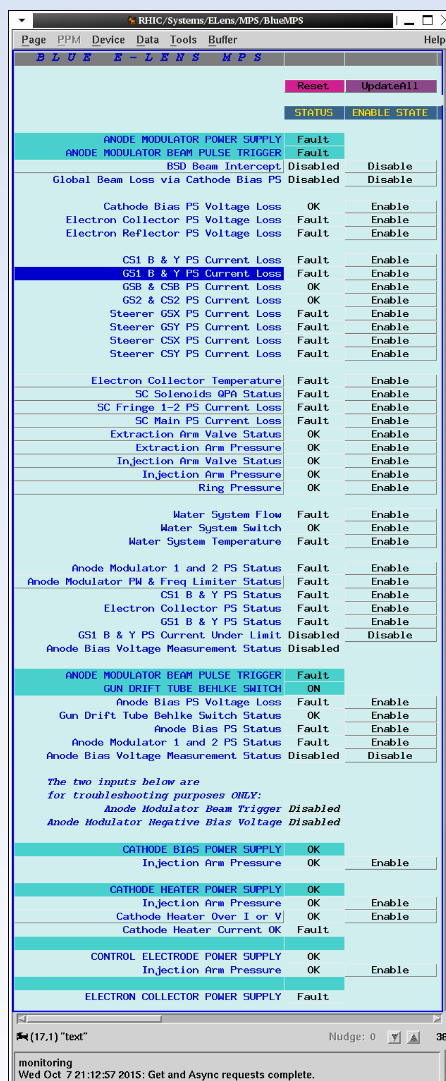
The Machine Protection System interface for the Blue e-Lens, showing a sampling of the current logic inputs and outputs.
