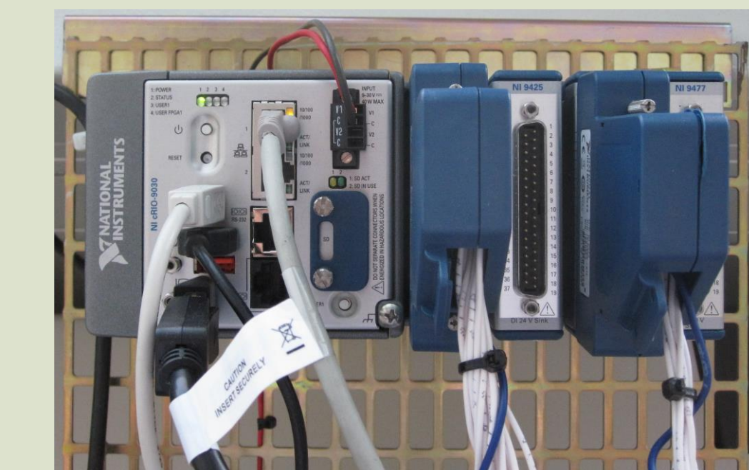
NI cRIO 9030 FPGA controller test bench. The RT-Linux unit is on the left and the FPGA unit on the right with I/O modules.
