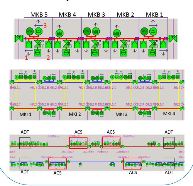
Interlocks are binary signals used within the vacuum system to prevent entering undesired states. They have a higher priority than the normal process logic or the operator's commands. Apart from the beam permit interlock, the vacuum control system does not interlock any other external systems directly.
