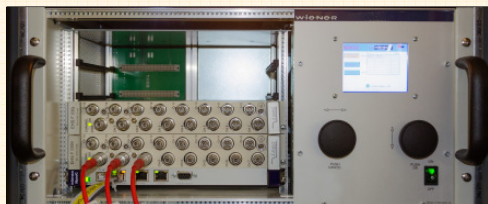
Wiener MPOD mini crate with four HV module slots. The lower slots are populated with 16-channel HV modules made by iseg.
