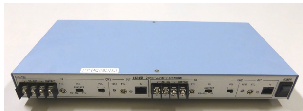
Figure 1: Picture of the 2ch E/O module. Input type and polarity can be set by slide switches (1424).
