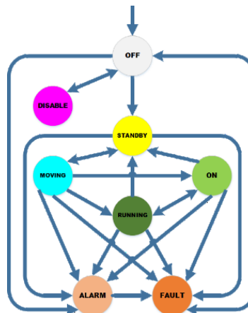
Figure 6: Power supply state machine in Tango view.
