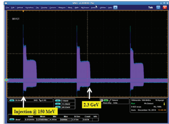
Figure 5: The beam loss occurred when beam ramping to 2.3 GeV observed on the first day of booster AC mode test.
