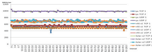
Figure 11: TCP/UDP test from kstar-s1 to ps and nfri-s1 and kstar-s2 after change.
