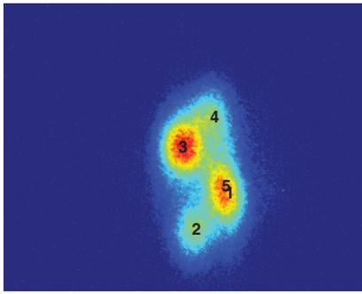
Figure 3: Superposition of 5 turns of stored beam during the injection kick with a 5 mA single bunch and no injected beam.
