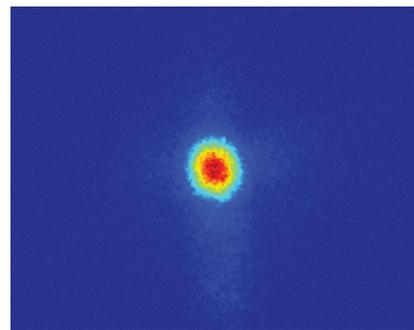
Figure 2: One turn of stored beam with a 5 mA single bunch in the ring.
