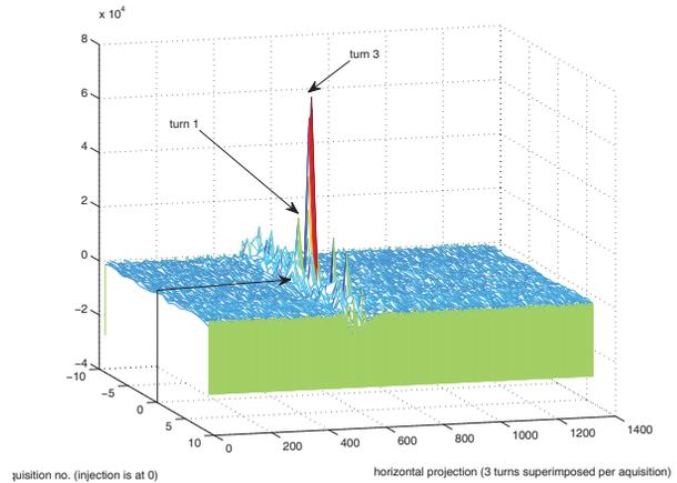
Figure 6: Waterfall plot showing the horizontal projection of each acquisition, with three turns captured per acquisition. The injection event is at acquisition point 0.
