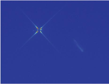
Figure 7: Image taken during the tuning of the coronagraph, great care must be taken to eliminate unwanted diffraction effects.
