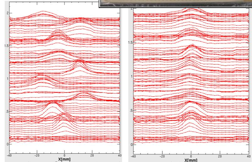
Results of injection beam orbit correction
