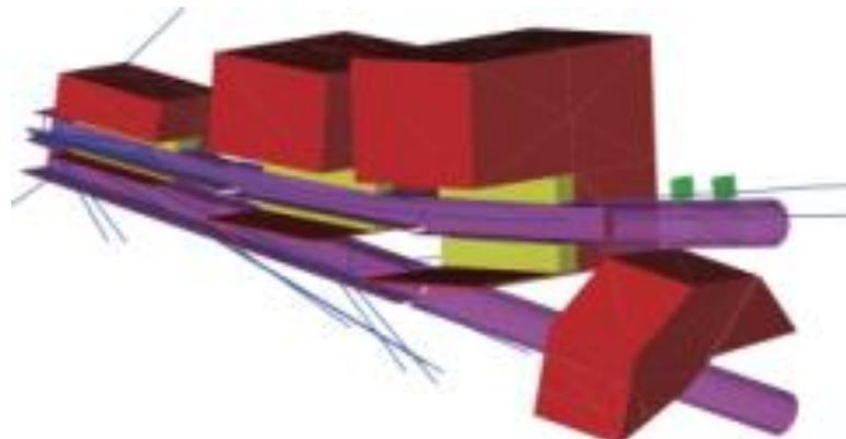
Estimation of scattered proton trajectory by G4BeamLine
