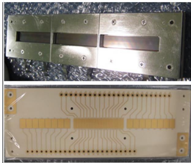
Figure 4: New MCP and anode plate.
