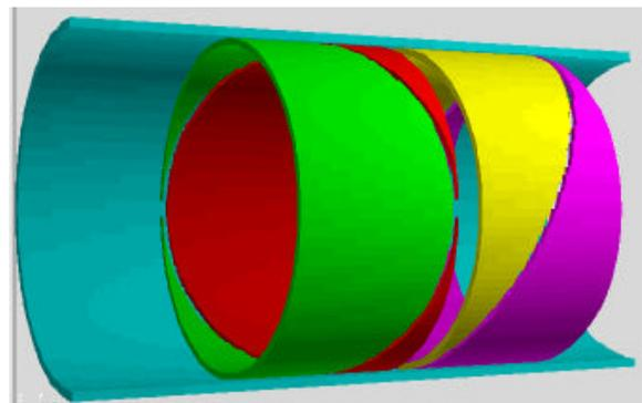
Figure 2: 3-D model of the diagonal cut electrodes.
