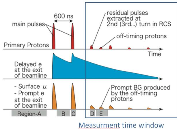
Figure 9: Measurement time window of DeeMe.
