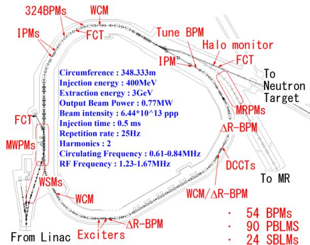
Figure 1: Monitor Layout and RCS parameters.
