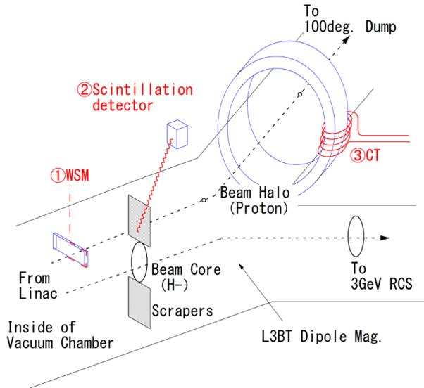
Figure 7: Schematic of the monitor system by the L3BT scraper.
