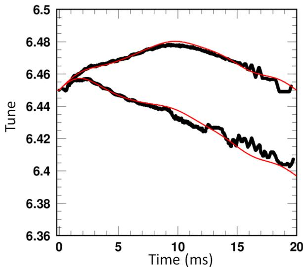
Figure 3: measured and calculated tune during acceleration. Black:measured, Red:calculated
