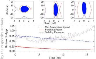
Figure 8: Phase space at the end of injection, 8.33 and 16.67 ms and evolution of bunching factor, stability parameter [8] and maximum dp/p.
