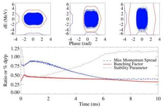
Figure 4: Phase space at the end of injection, 5 and 10 ms (top), evolution of bunching factor, stability parameter, peak dp/p for proposed injection scheme (bottom).
